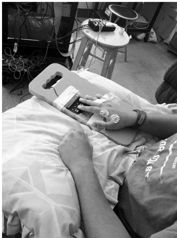
Fig 1. A custom keyboard was developed to allow the index finger to reach the 7, 8, and 9 keys of the numeric keypad. Other digits were then taped down to allow the proper hand orientation to enable the index finger to move freely and optimally activate the FDI muscle through abduction. Recording electrodes placed over FDI are also shown.
